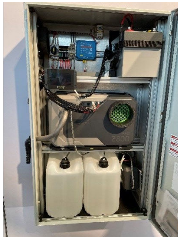
Methanol based and hydrogen-based electricity generators, designed for extreme cold.
